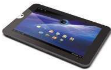
Thrive tablet has two USB ports, uploads photos, connects to TV.
